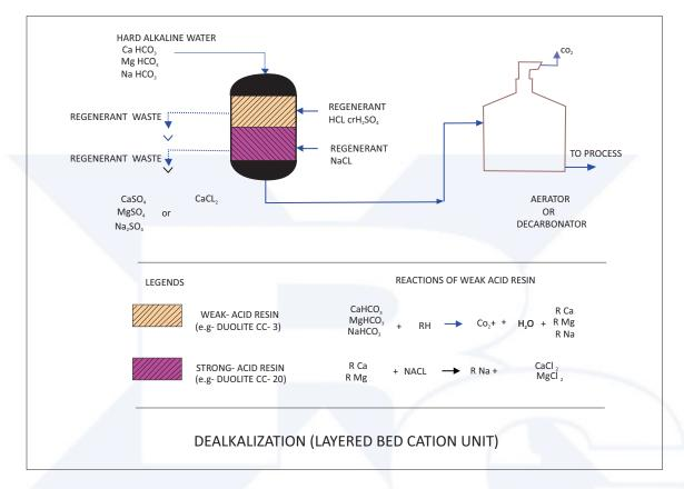
Note that the dealkalizer would seldom be used without a base-exchange softener, as the solution produced is acidic and would cause corrosion, and any permanent hardness would straight into the boiler.
